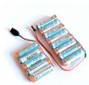
Battery pack for the radio, system and servos' working
