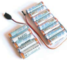
Battery pack for the radio, system and servos' working
